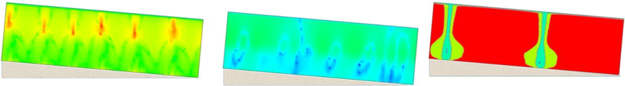
Fig. 2c: Contours of curvature at 6000 s from left to right for:  $Ri = 0.06, 0.2$  and  $0.3$ . The maxima of this field correspond to critical points.
