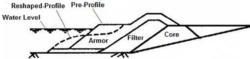
Fig. 4: physical modeling of berm reshaping seawall
