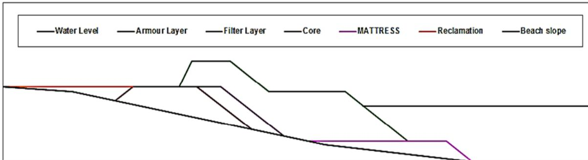
Fig. 1: Berm reshaped seawall
