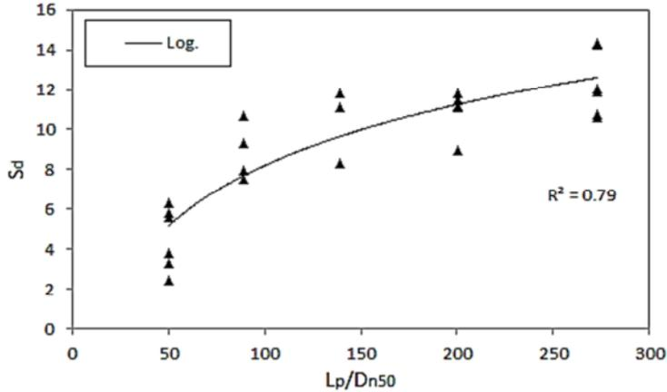
Fig. 6: damage parameter diagram against maximum length wave
