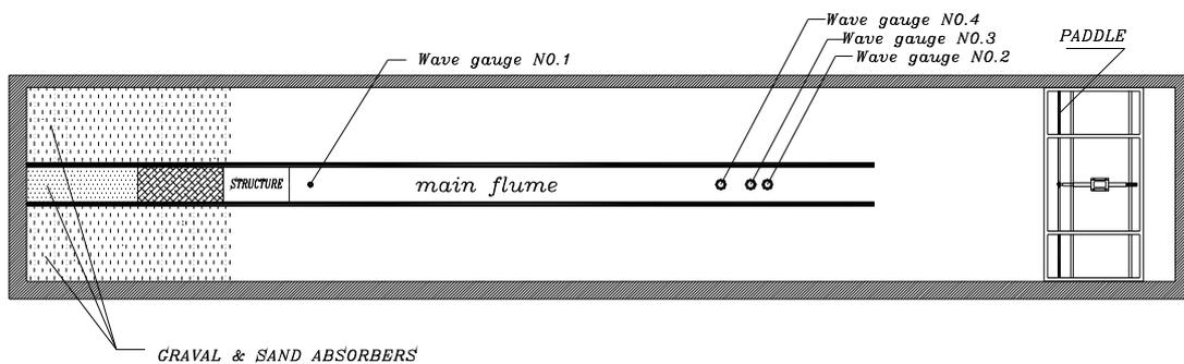
Fig. 2: Plan view of the wave flume and setup of wave height meters
