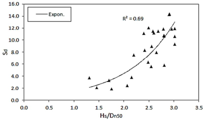
Fig. 5: damage parameter diagram against significant wave height
