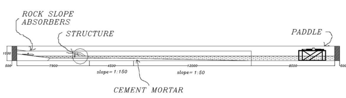
Fig. 3: Cross section of the wave flume
