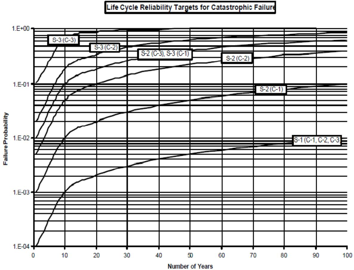
Fig. 5: Life cycle reliability target for catastrophic failure
