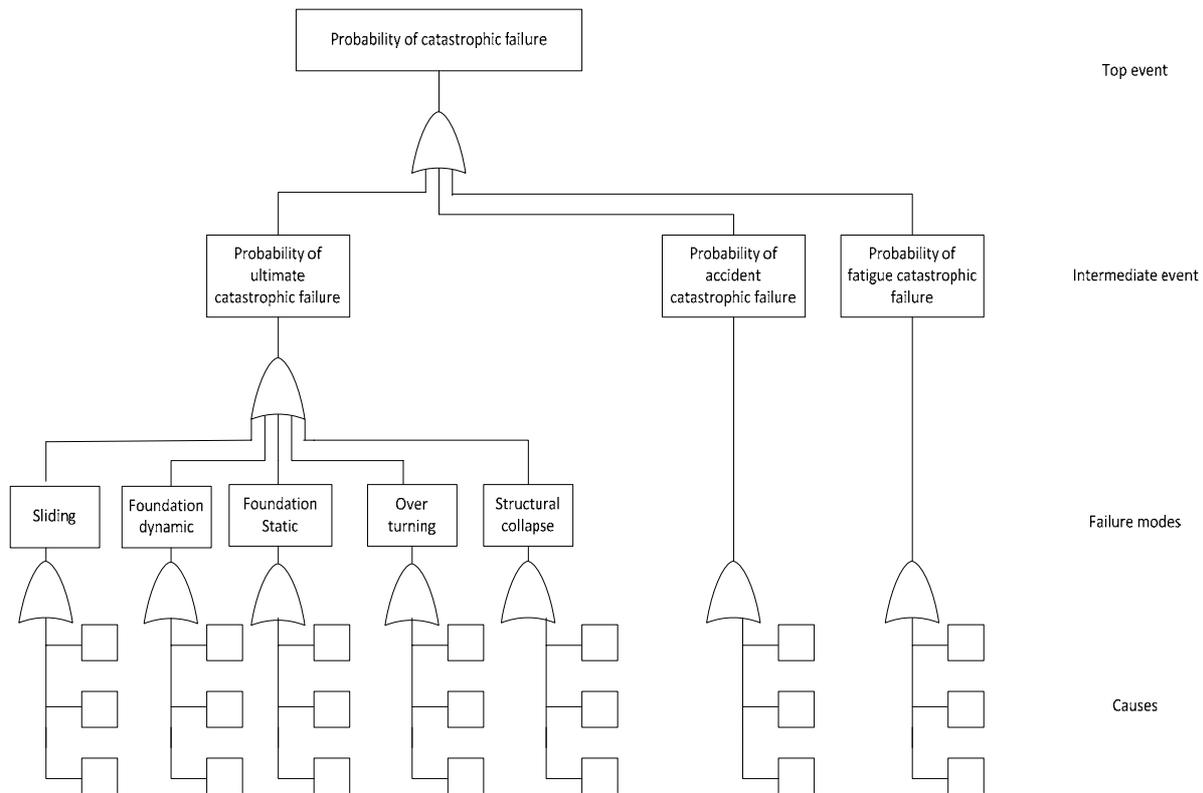
Fig. 4: Catastrophic failure fault tree
