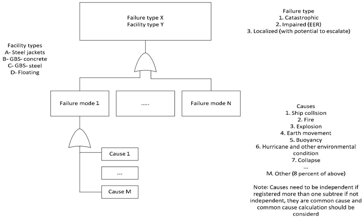
Fig. 3: Offshore structures generic fault tree
