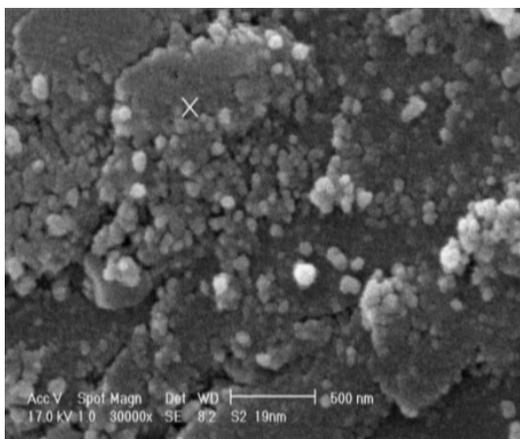
Fig. 5: SEM image of TiO<sub>2</sub>/SiO<sub>2</sub> thin film sample
