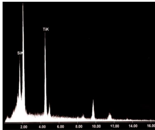
Fig. 6: EDX image of TiO<sub>2</sub>/SiO<sub>2</sub> thin film sample
