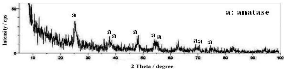
Fig. 2: XRD pattern of  $\text{TiO}_2/\text{SiO}_2$  thin film sample
