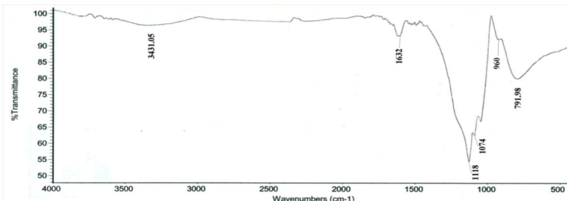
Fig. 4: FT-IR spectrum of TiO<sub>2</sub>/SiO<sub>2</sub> sample
