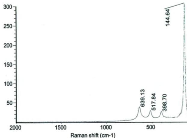
Fig. 3: FT-Raman spectrum of TiO<sub>2</sub>/SiO<sub>2</sub> sample
