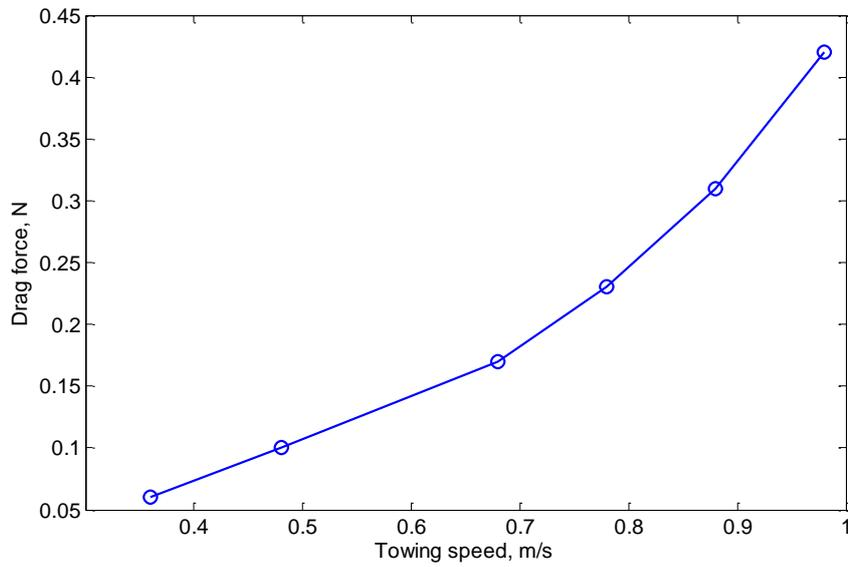
Fig. 7: Resistance curve vstowing speed for a benchmark displacement vessel
