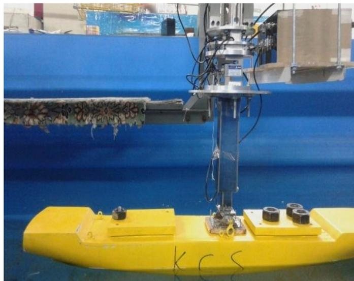
Fig.6: View of the dynamometer and model under towing carriage
