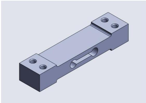
Fig.4: load cell to measure bending force
