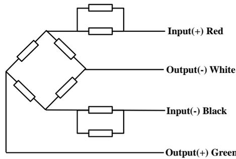
Fig. 3: An example of the strain gauge wheatstone bridge arrangement
