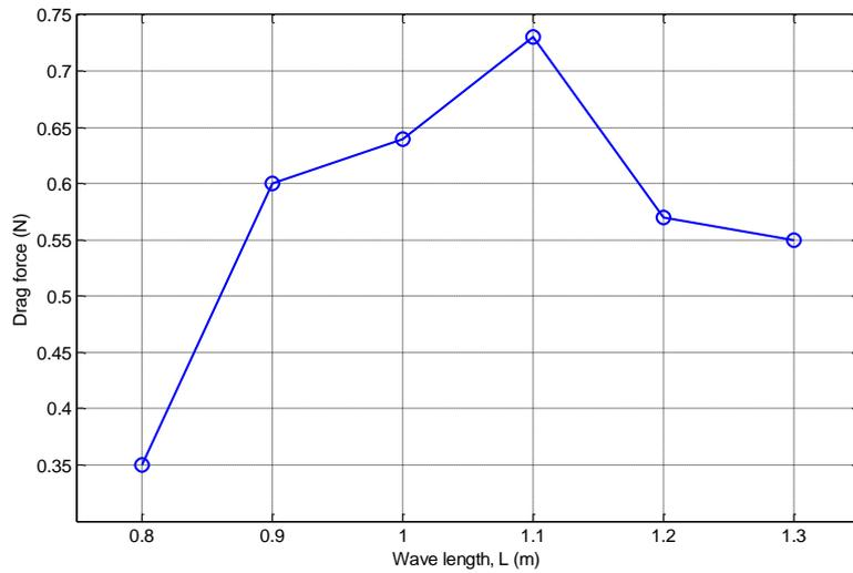
Fig. 8: The resistance curve of a displacement vessel with different wavelength with a constant speed of 0.64m/s and wave amplitude 2cm
