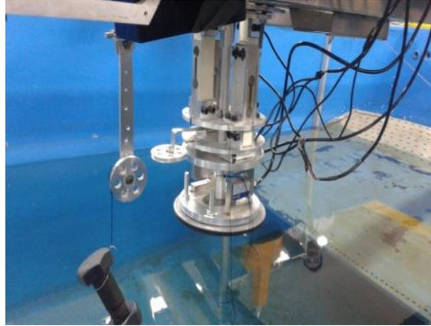
Fig.5: View of sensor calibration for drag force
