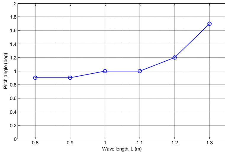
Fig. 9. The maximum pitch angle of a displacement vessel with different wavelength with a constant speed of 0.64 m/s and wave amplitude 2 cm
