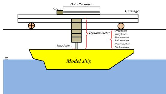
Fig. 1: Side view of the towing tank, model, systems and dynamometer operation
