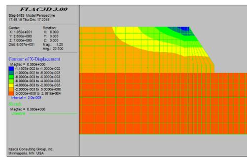
horizontal displacements in Inclined wall
