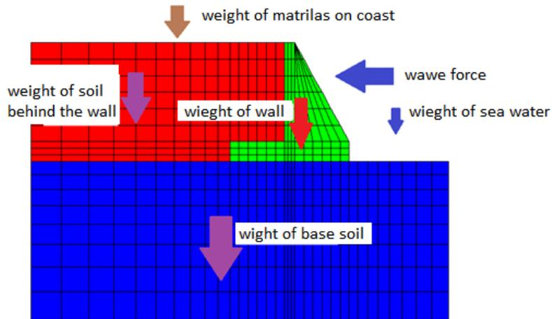
Fig. 2: Schematic forces on seawall
