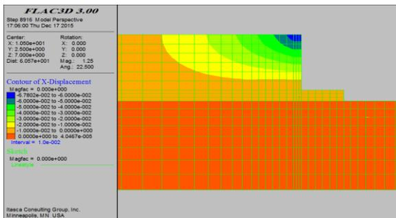
horizontal displacements in vertical wall
