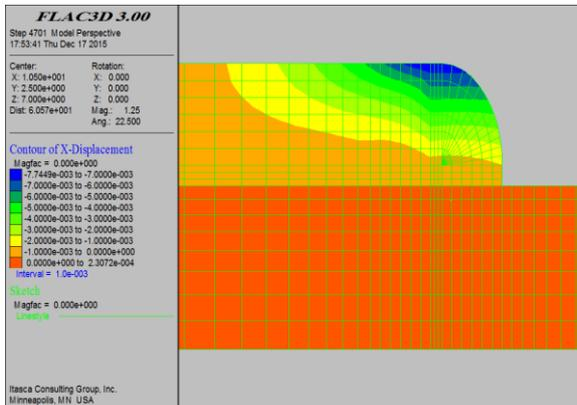
horizontal displacements in Convex wall
