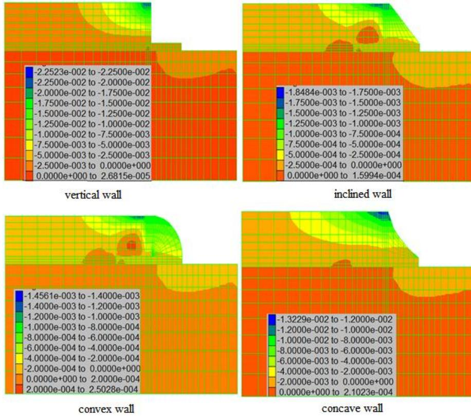
Fig. 6. the amount of horizontal displacements in different walls
