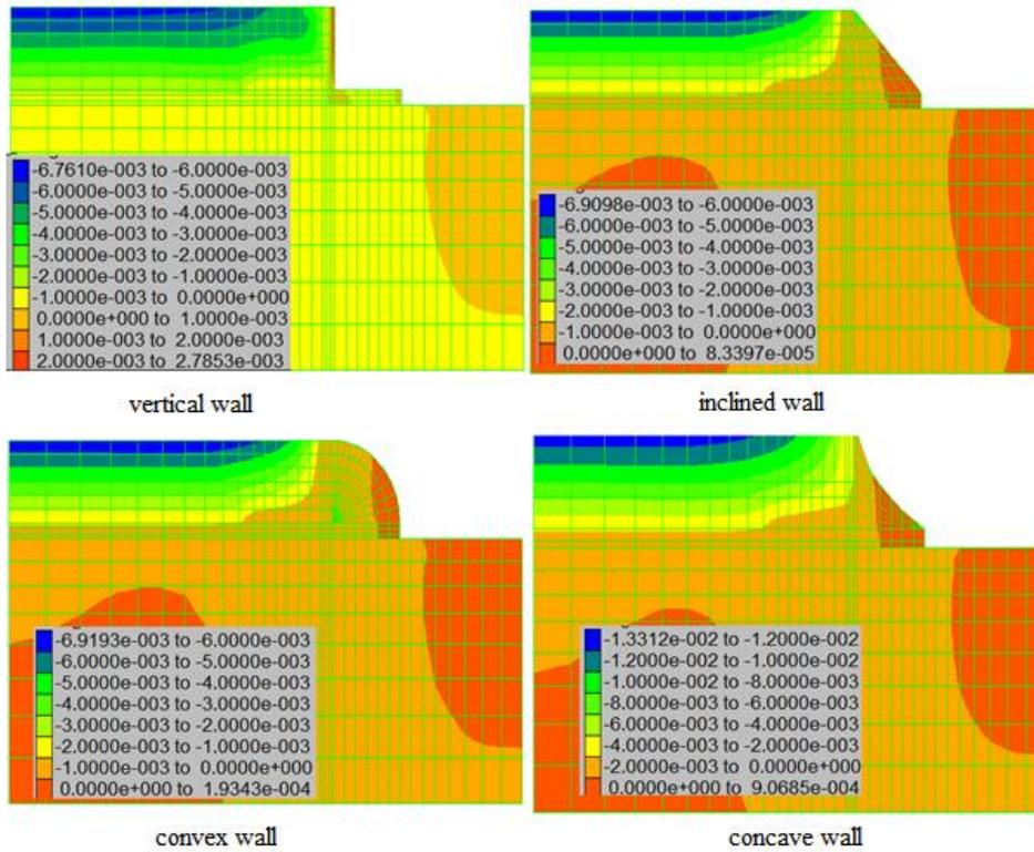
Fig. 7: Amount of vertical displacements in different walls
