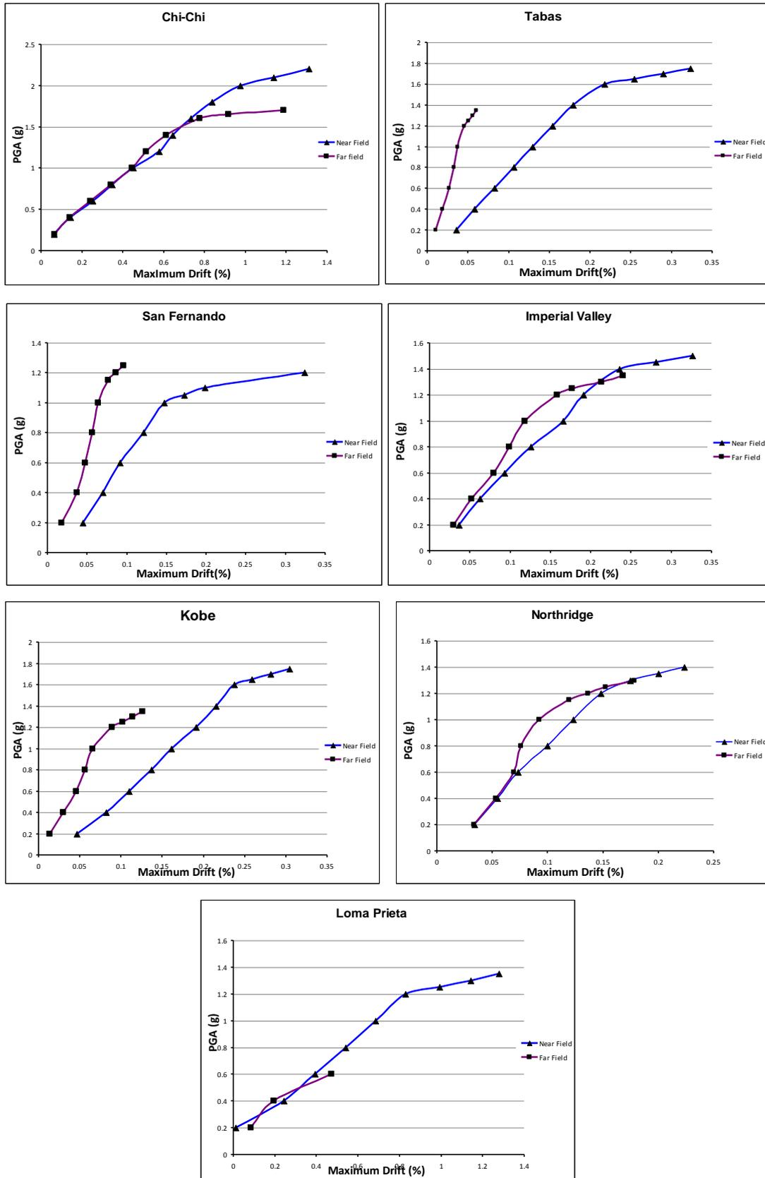
Fig 7: Near & Far- fault comparing IDA diagram at different sites
