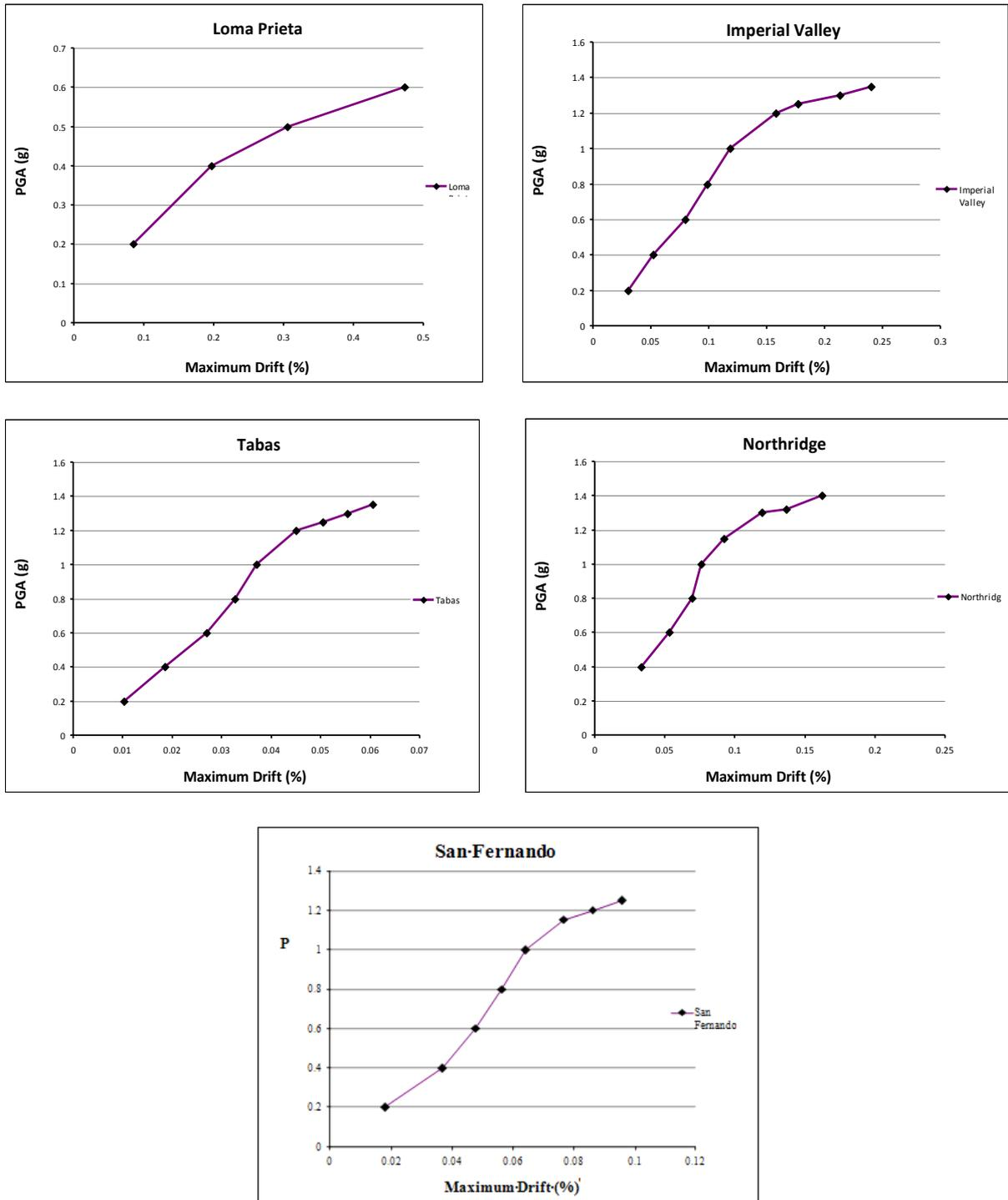
Fig. 6: Far-fault records-IDA diagram at different sites
