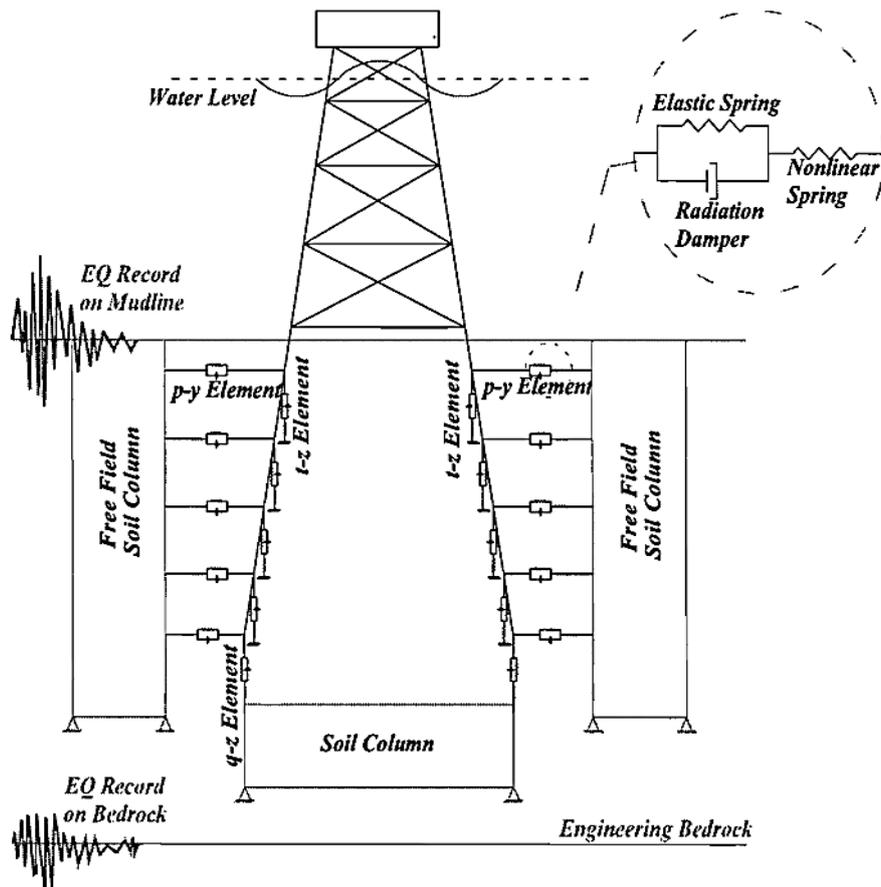
Fig. 2: Modeling of soil-pile structure interaction
