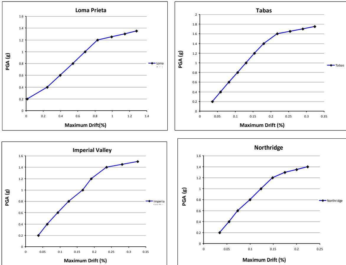
Fig. 5: Near-fault records-IDA diagrams at different sites
