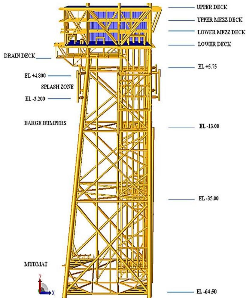
Fig. 1: Isometric view of SPD 19 Platform
