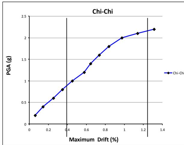
Fig. 4: Near-fault record- chichi IDA diagram
